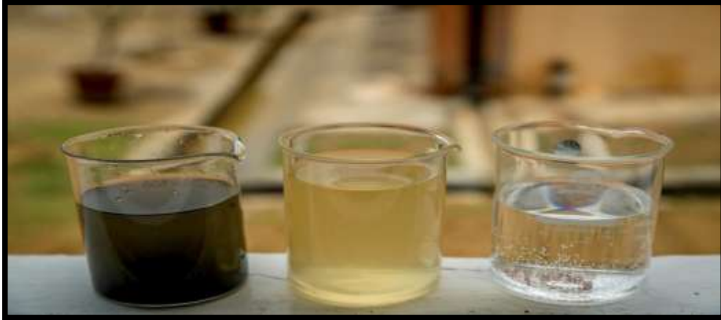
Figure 4: showing Raw Sewage, After Bio-Filter and After Membrane quality water
